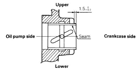
2) Bearing metal on motor side.
